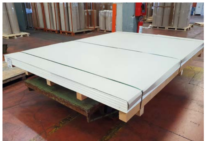
Made-to-measure standard pallet with continuous wooden surface
